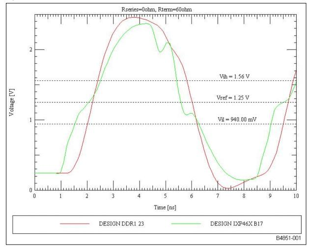
Figure 46. DDR Address Simulation Results: Two-Bank x16 Devices
